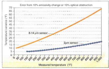
Short-wavelength IR sensors are not as sensitive to changes in emissivity on the target material as conventional, high-temperature sensors.
