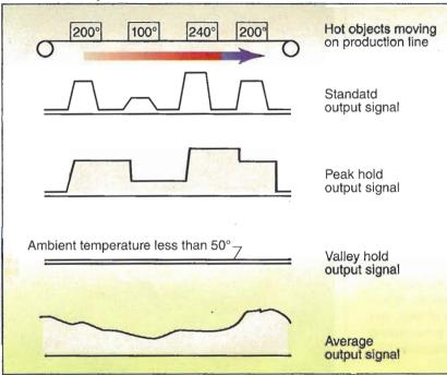
Innovations in IR sensor electronics have also improved signal processing capabilities, including emissivity, sample and hold, peak hold, valley hold, and averaging functions.
