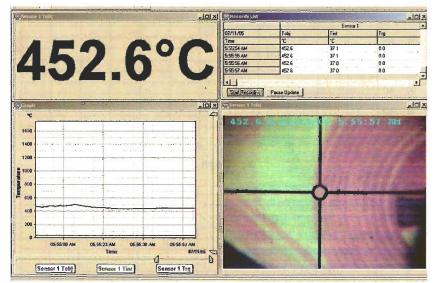
A system combining noncontact infrared temperature measurement and data acquisition software can control a set-point temperature.
